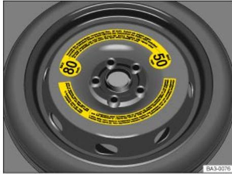
Fig. 94 In the luggage compartment: Compact spare wheel.
