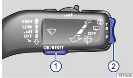
Fig. 15 Basic version (vehicles without menu control multi-function steering wheel): Control buttons 1 and 2 on the windshield wiper lever.
