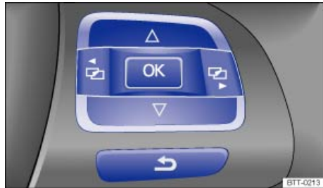
Fig. 16 Premium version (vehicles with menu control multi-function steering wheel): Buttons on the right side of the steering wheel.
