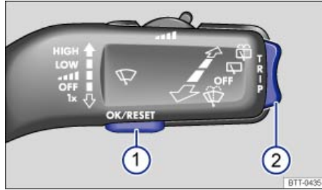
Fig. 17 Premium version (vehicles without menu control multi-function steering wheel): Control buttons 1 and 2 on the windshield wiper lever.
